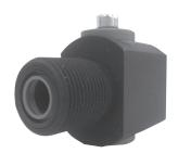
Series of piston rod brakes rod units for cylinders ISO 6432 with pneumatic releasing and rod mechanical locking obtained through a double jaw (the locking is pneumatic in the type normally open).
